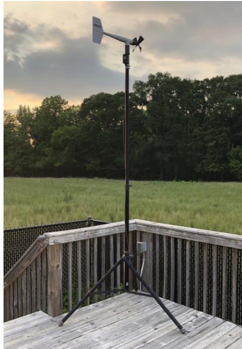
Figure 1. Wind Speed and Wind Direction Monitor
